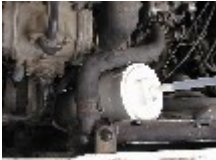
This is an installed test fit, again checking for hood clearance
